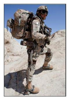
Figure 3. The Lockheed HULC. Photo courtesy of Lockheed-Martin.
